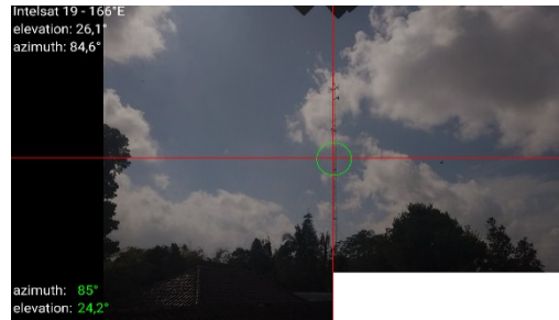
Gambar 6. Posisi pointing satelit Intelsat
